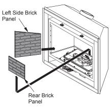
Figure 39 - Installing Rear Brick Panel
